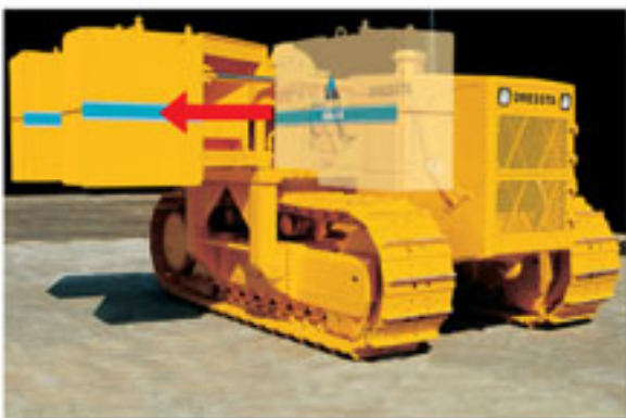
Extendable and retractable counterweights
